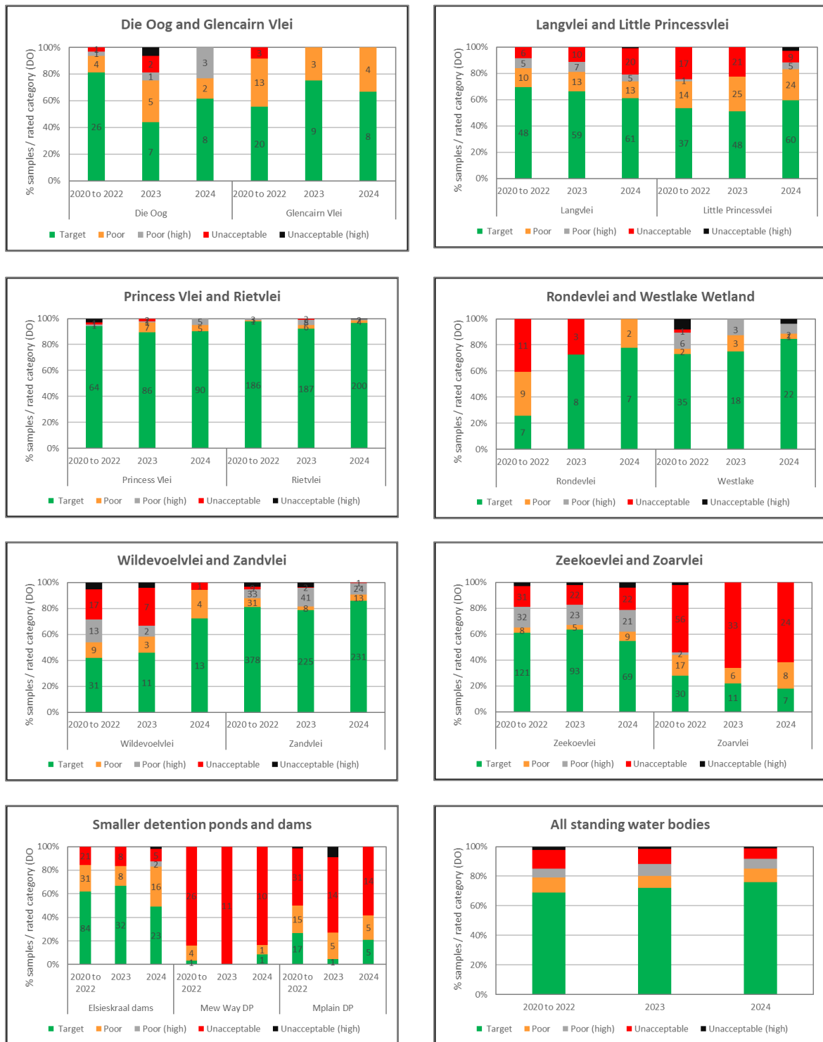
Figure 5.5.4 Percentage of samples falling within each rated category for Dissolved Oxygen (DO), per monitored standing water system for Reporting Years 2020-2022, 2023 and 2024. Thresholds for rated categories as defined in Table 3.3. Total number of samples considered shown in bars of each plot.
